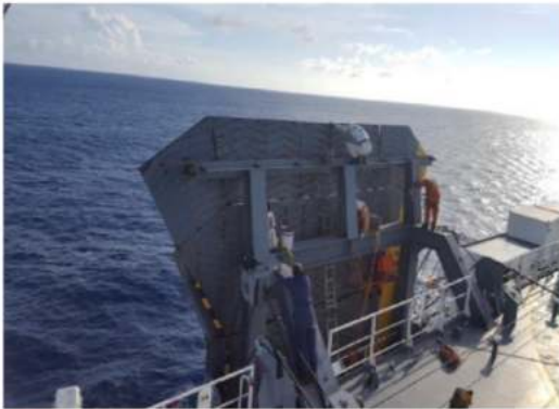
Surface preparation - high pressure water
